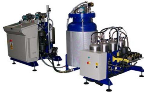
CTM EP 60 Epoxy dispensing machine
